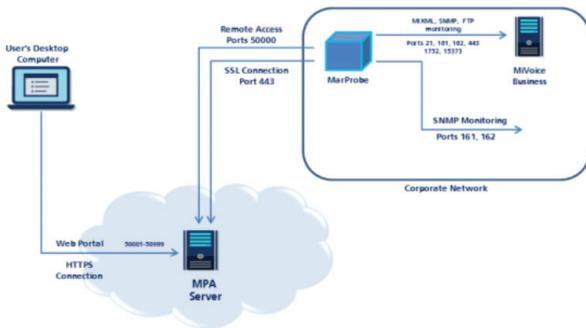
**Remote Access Control Settings:** Mitel Performance Analytics provides controls for the Remote Access feature through the Probe Settings page. Users can configure the Probe to:
