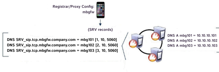
Figure 2: DNS SRV Entries for Resilient Softphones in Cloud Deployment
