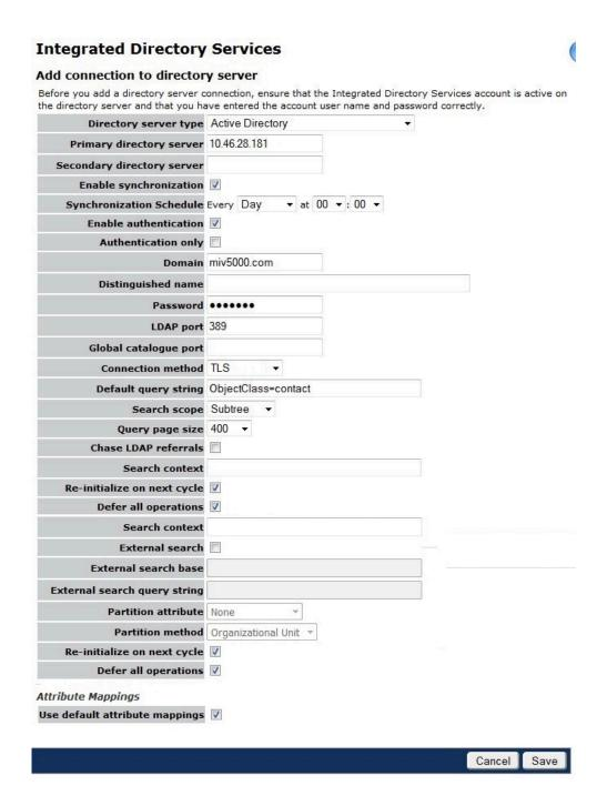
Figure 1: IDS Connection for MiVoice 5000 with Contacts from Active Directory
