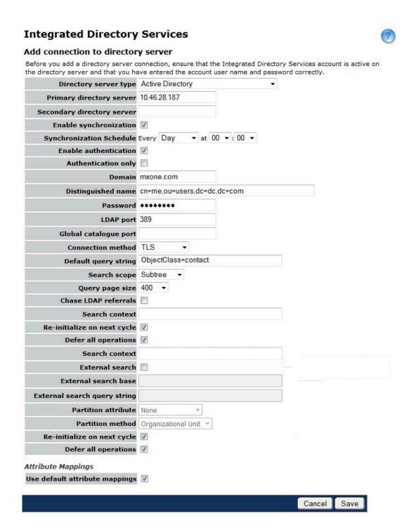
Figure 1: IDS Connection for MiVoice MX-ONE with Contacts from Active Directory
