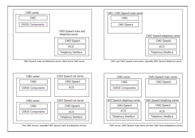
Figure 1 Possible CMG Speech Installation Configurations
