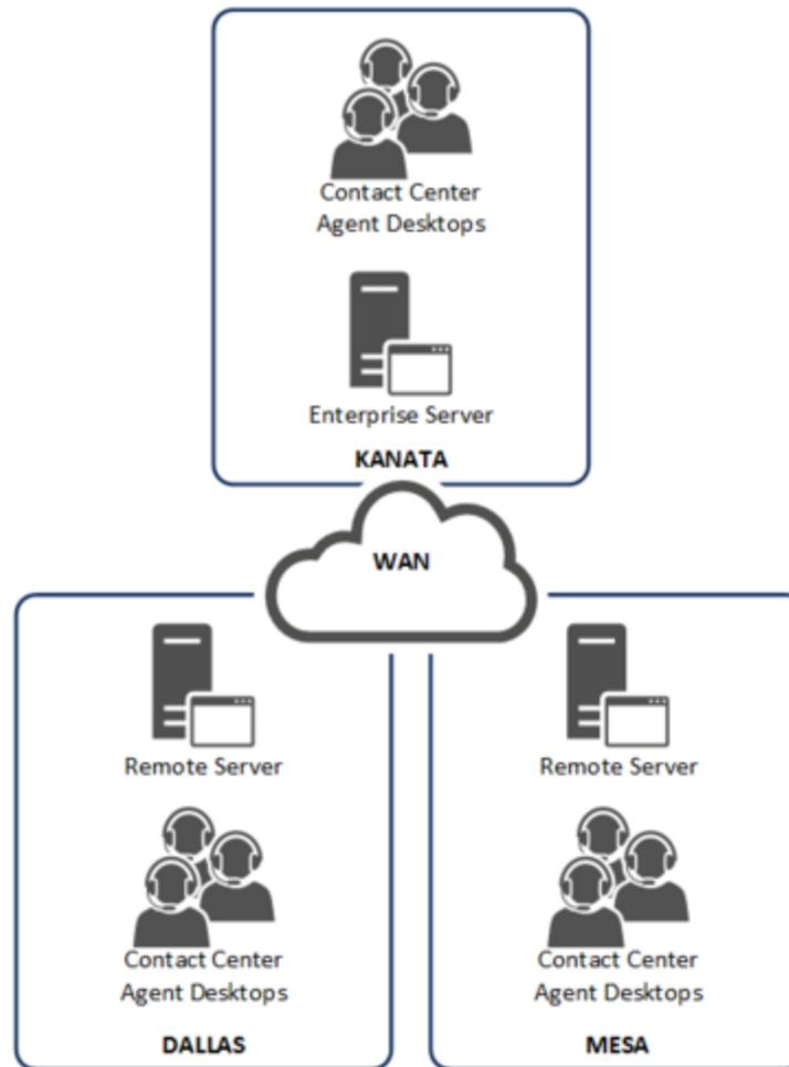
Figure 1: Sample distributed contact center with remote servers handling client updates
