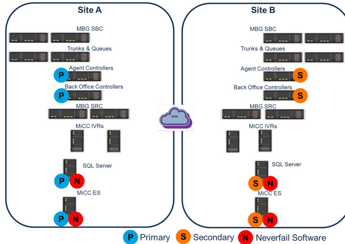
Figure 5: Disaster Recovery deployment model
