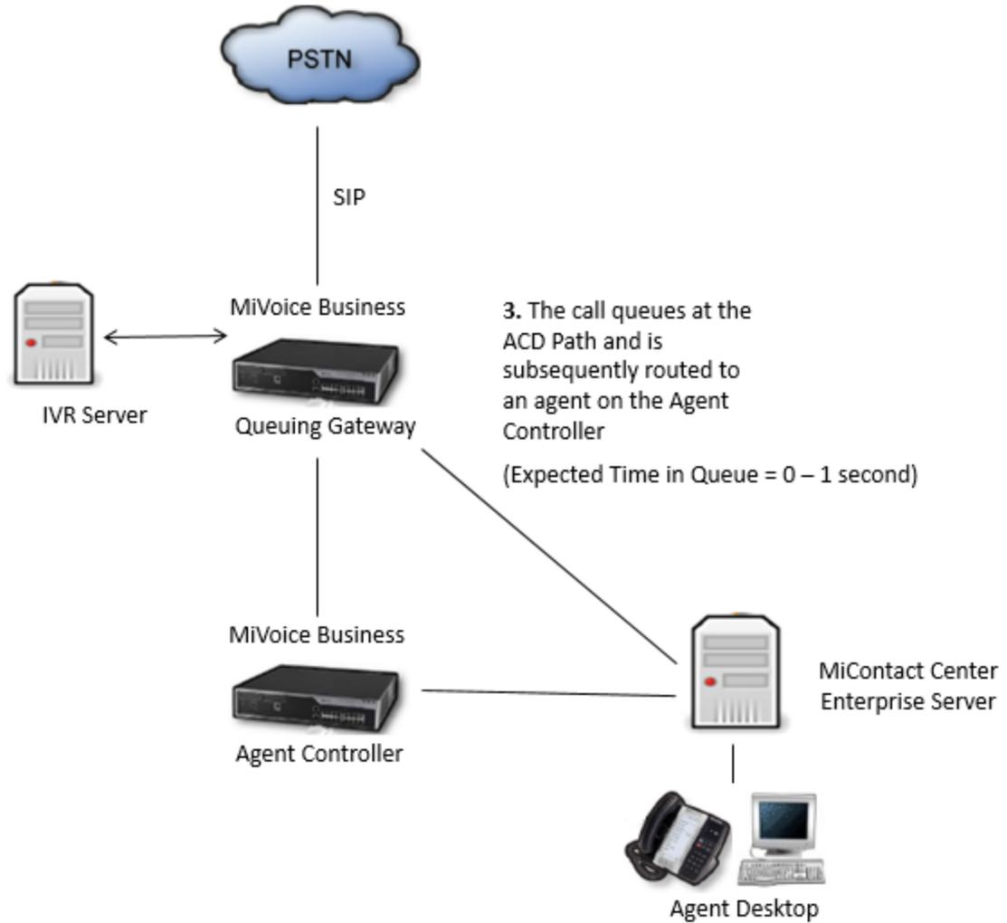
Figure 10: Verification environment call flow with IVR Routing
