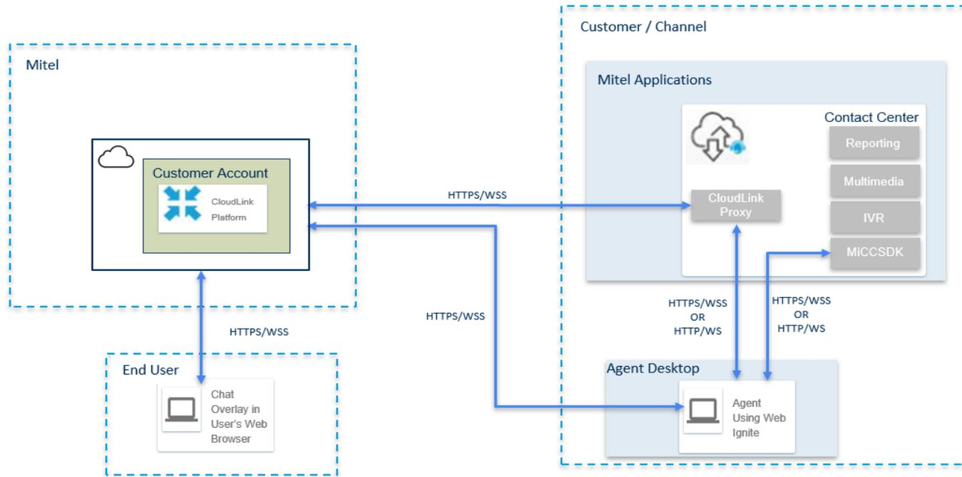
Figure 18: Contact Center Messenger Chat Integration when not configured to use Google AI features
