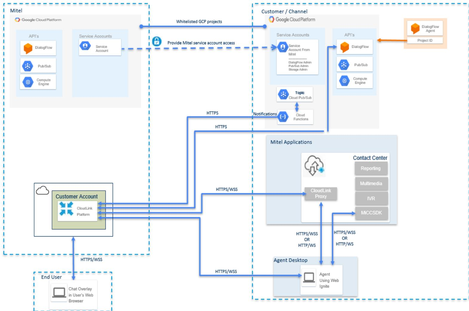
Figure 19: Contact Center Messenger Chat integration when configured to use Google AI features
