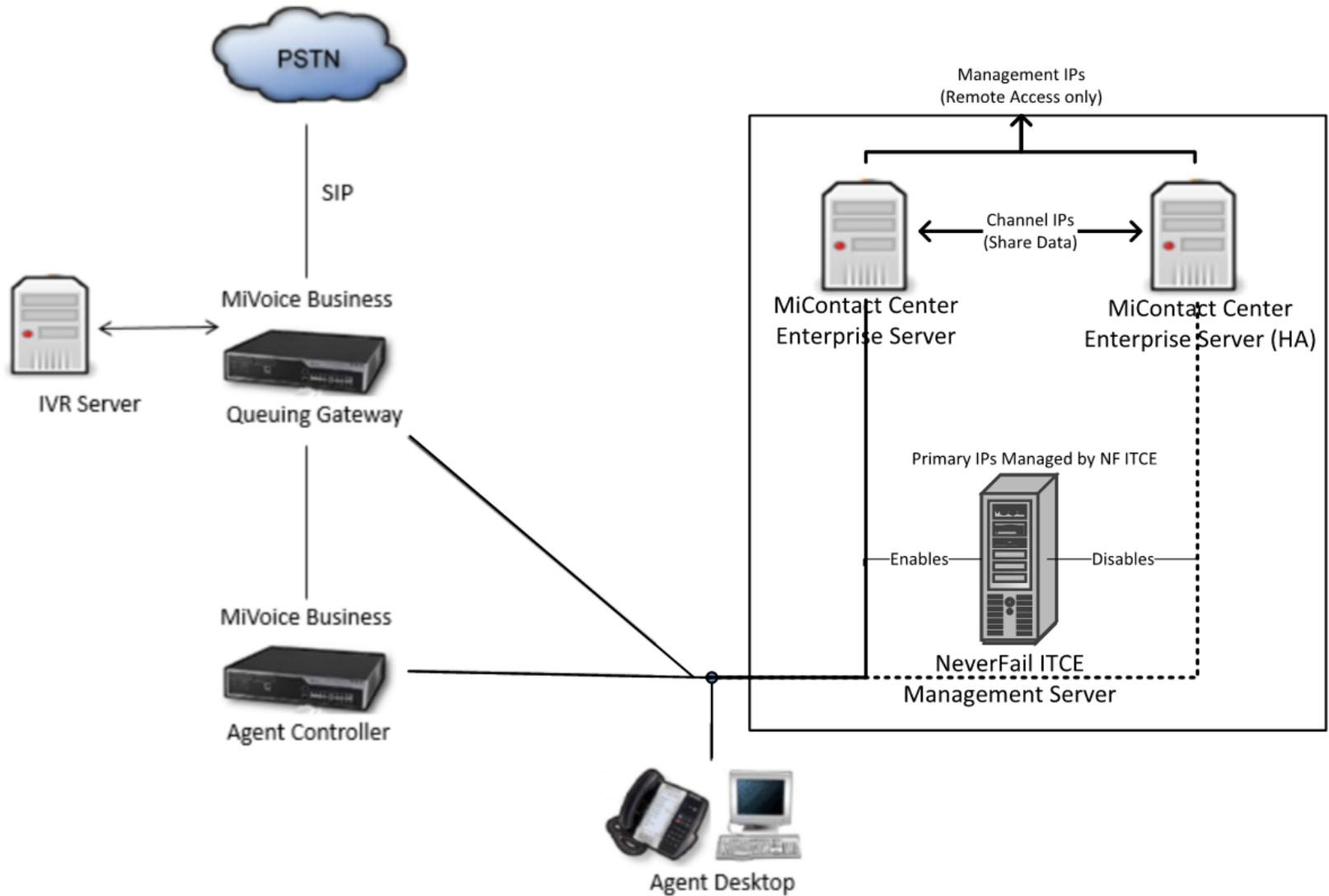
Figure 12: HA verification topology for voice media capacity with or without IVR routing
