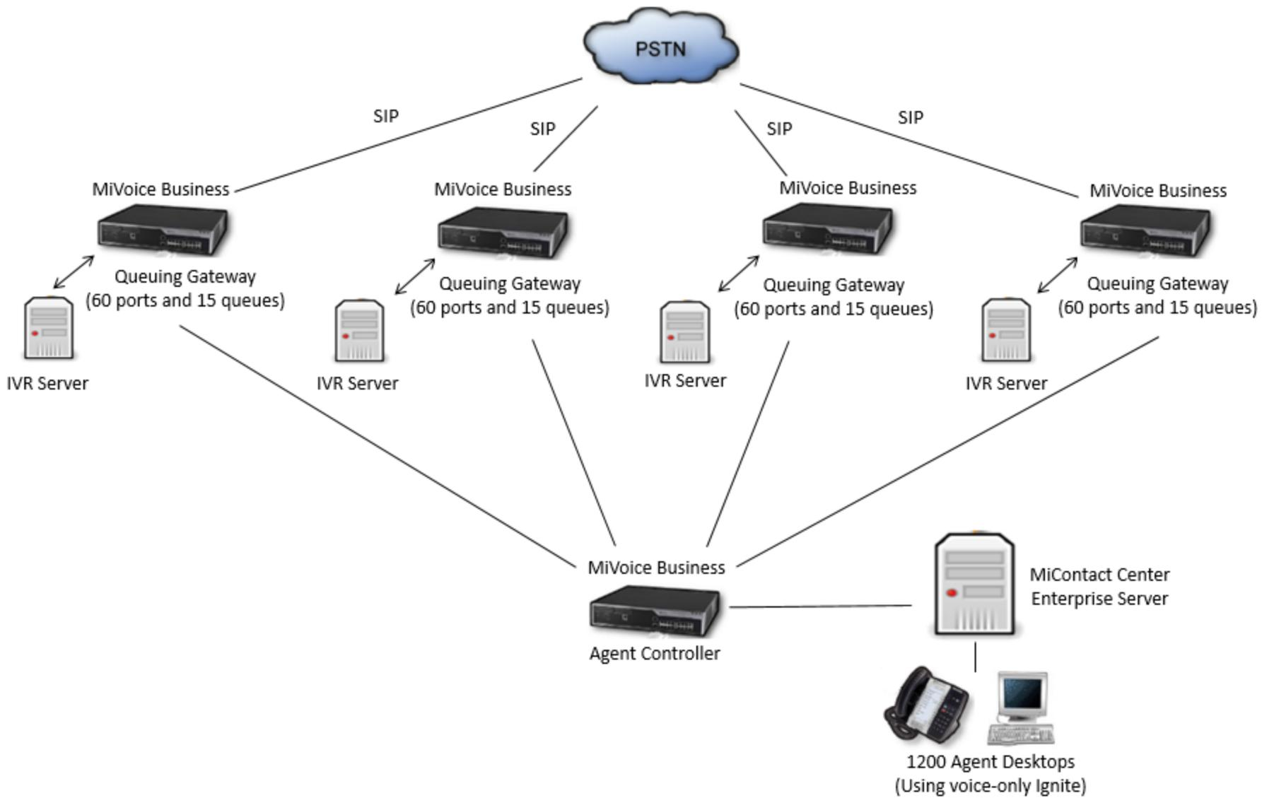
Figure 9: Verification environment with IVR Routing
