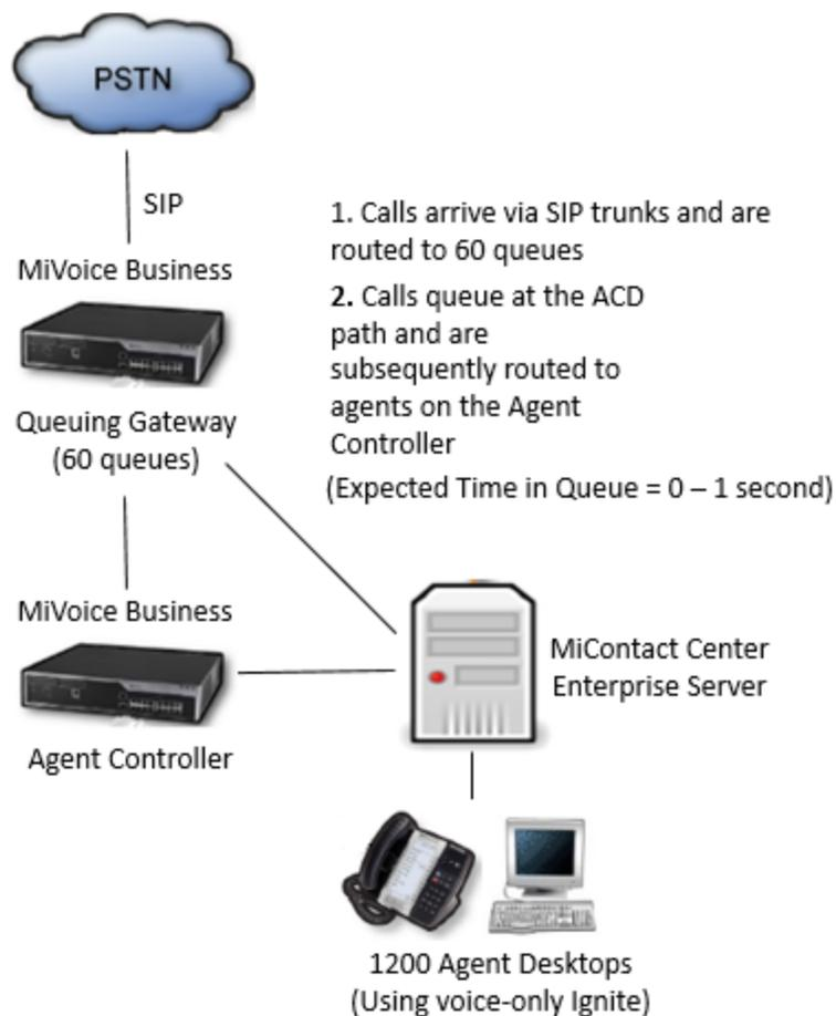
**Figure 8: Verification environment and call flow – with MiVoice Business routing (no IVR)**
