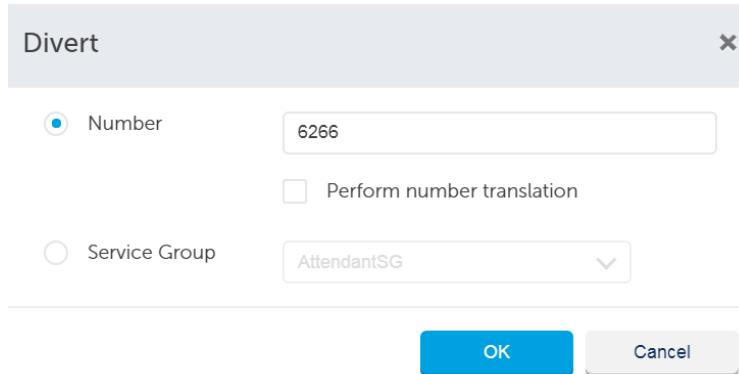
Enter the number to which the voice call should be diverted in the *Number* field. If Number Translation parameters are configured in the MiCC-E system parameters, the *Perform Number Translation* option is enabled. Checking this option applies the defined number translation rules to the number before dialing. For example, an access code to dial out can be prepended to the number.
