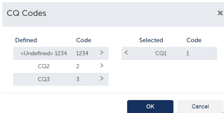
Select any defined call qualification codes from the *Defined* list and press the *>* button to move the code from the *Defined* to the *Selected* list. To remove a call qualification code, press the *<* button to move the code back to the *Defined* list. The selected call qualification codes will be associated with the service group session.
