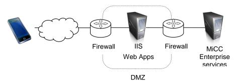
In this architecture however, multiple connections must be allowed between this server and the other MiCC Enterprise server(s) located in the LAN.
