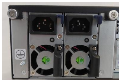
Figure 9: OSB 550HA-Redundant AC Power Supply 2x300W (high availability)
