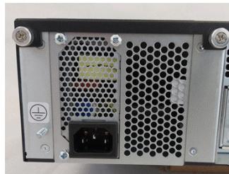
Figure 8: OSB 550- PSU 300W AC with single AC input power socket
