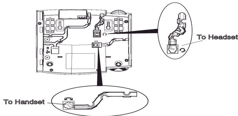
Figure 2 Handset/Headset Connection
