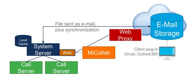
The MiCollab Advanced Messaging functionality is provided by the System Server and a number of Call Servers. The scaling of these is described in a following section.
