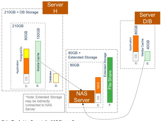
Server H is similar in operation to the Server A (All-in-One) except that recording is carried out on a different server. This server still requires the media cache as this will still need to carry out a number of post recording tasks. Although the separate Data HDD is identified as HDD, and will work as HDD, the recommendation for these larger servers is to use SSD where possible.
