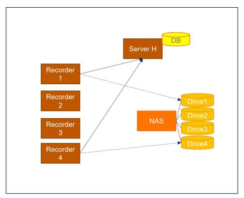
In this example there are 4 recorders and each points to a specific drive associated with this recorder. Each recorder still connects to the core server (H) in order to update the database.
