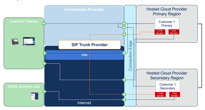
(Not all possible connections are shown to simplify the diagram, for example, the customer premises will connect over the Internet to both primary and secondary user MiVoice Border Gateways, and similarly the SOHO/Nomadic users will connect to both primary and secondary MiVoice Border Gateways.)
