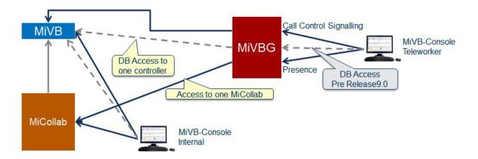
The internal MiVoice Business Console connects directly to the associated MiVoice Business Controller for Call Control Signaling. It connects directly to the associated MiCollab Client Presence Server. In addition, there is an optional connection to the MiVoice Business Controller for database access. The link is only required for backward compatibility to MiVoice Business prior to Release 9.0.
