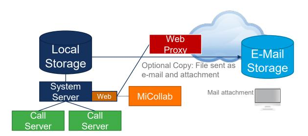
The MiCollab Advanced Messaging functionality is provided by the System Server and a number of Call Servers. The scaling of these is described in a following section.
