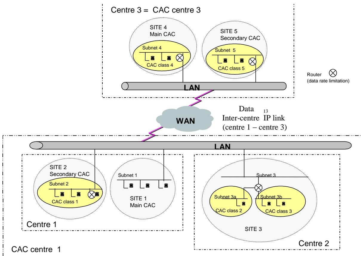
Figure 2: Managing CAC in a multi-centre, multi-class configuration
