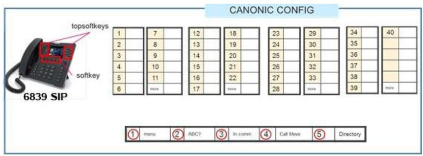
**Note :** The 3 expansion modules M680i are used to manage up to 48 additional programmable keys.
