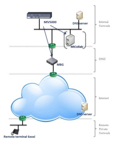
The aim is for a remote 6800 SIP or 6900 IP phone to have almost the same functions as a similar phone installed on the company's local area network.
