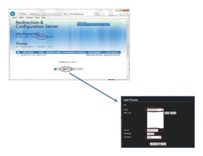
The remote station, after a factory reset (in SIP mode) will connect to the RCS server and automatically retrieve the address of the MBG associated with the iPBX in question.
