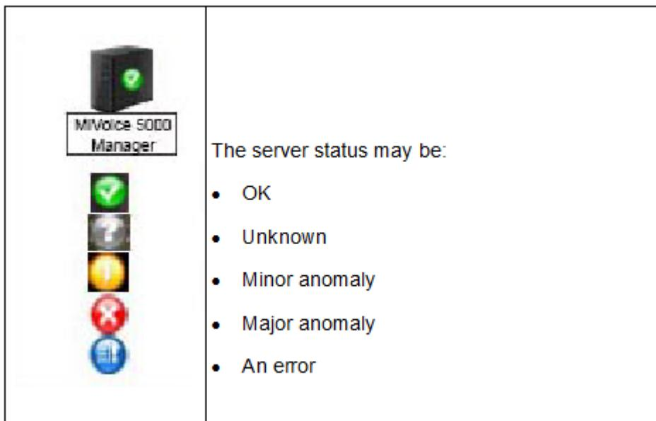
Placing the cursor over the MiVoice 5000 Manager symbol displays its characteristics as well as the status of the different associated services:
