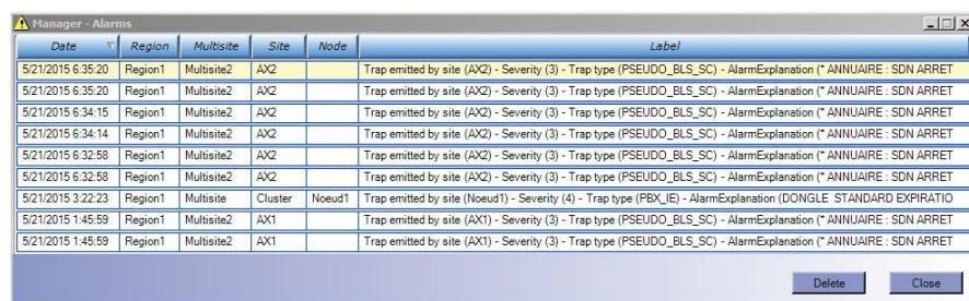
The **Delete** button is used to delete a selected alarm line from the display window. The event is, however, preserved in the MiVoice 5000 Manager database.
