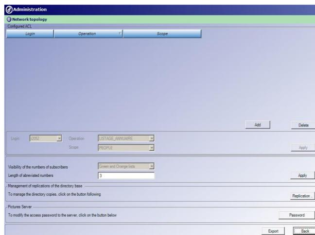
This window allows you to configure external applications' access rights for the LDAP directory. A login is created for each application. These logins have already been defined in the **Configuration** part.
