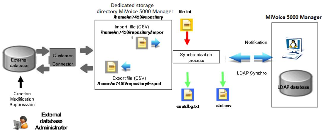
The principle is to synchronise the external directory database and the MiVoice 5000 Manager LDAP database by exchanging description files in **UTF-8 without BOM**.
