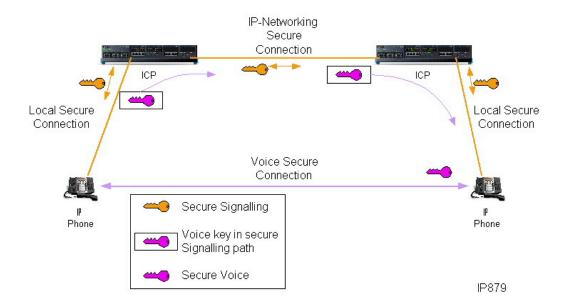
Figure 45: Media and Signalling Path Encryption
