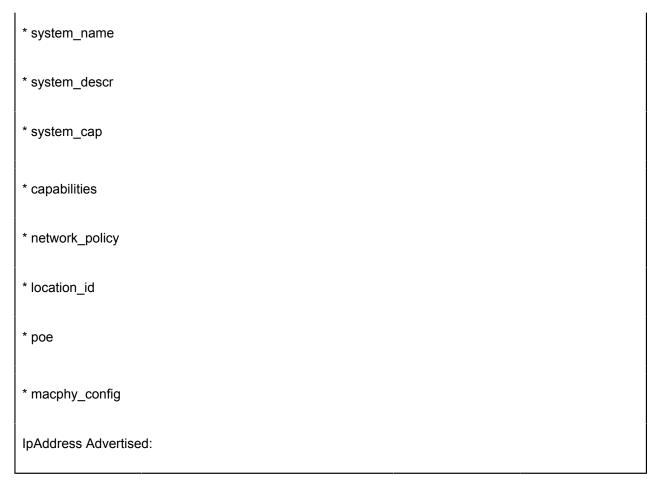
The capabilities option and network policy are both needed for auto configuration of the end devices.
