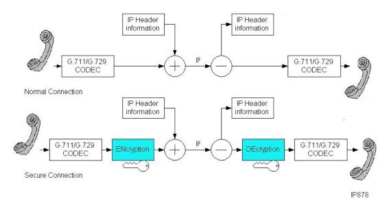
Figure 44: Unsecured vs. Secured Connection
