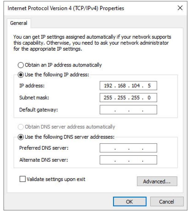
Figure 29: Configuring Programming PC to SMB Controller Default Subnet
