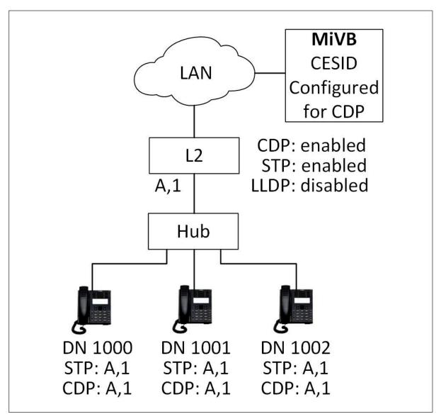
Figure 15: Non-compatible Network Configuration - Devices Connected via Hub
