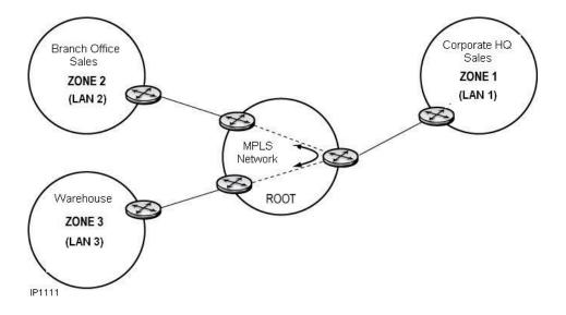
Figure 22: Fully-meshed WAN Connections - Star Configuration
