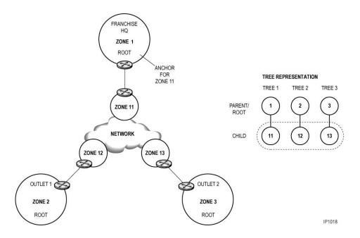
Figure 24: Topology for Non-meshed Configuration
