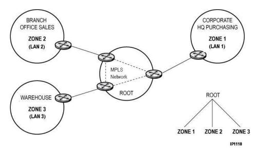
Figure 21: Fully-Meshed WAN Connections - Deployment Example
