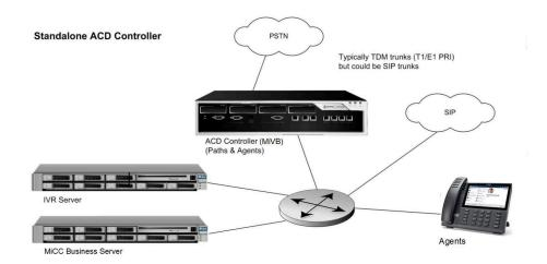
Figure 6: Example of a Standalone ACD Installation
