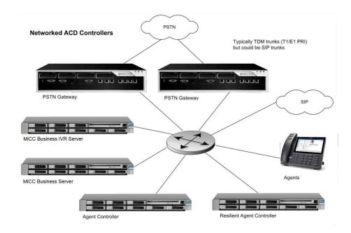
Figure 7: Example of a Networked ACD Installation
