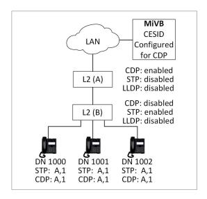
Figure 14: Non-compatible Network Configuration - L2 Switch - CDP and STP Disabled
