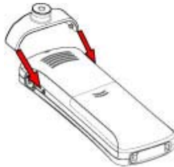
Figure 12: Click the clip into position
