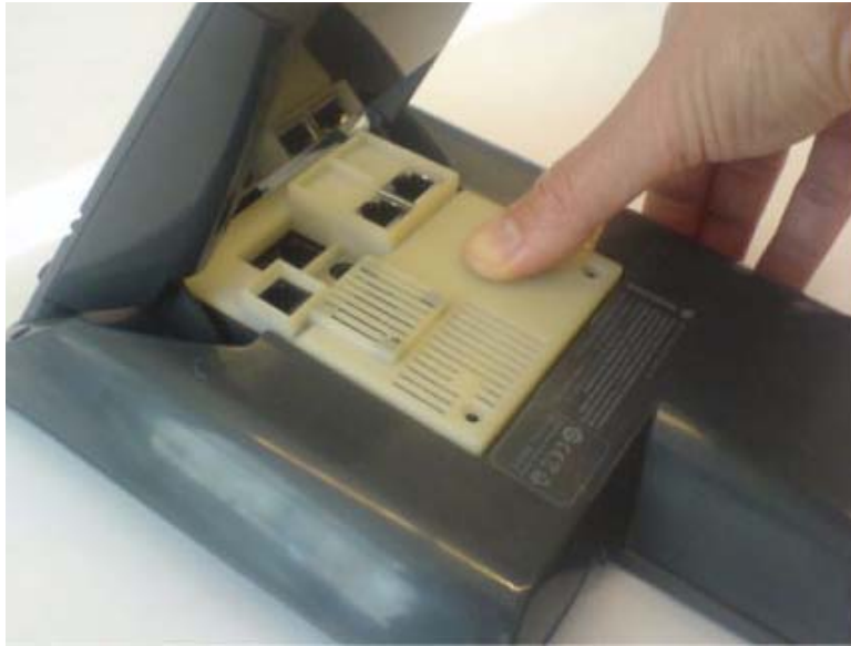
Figure 18: Attaching the option unit
