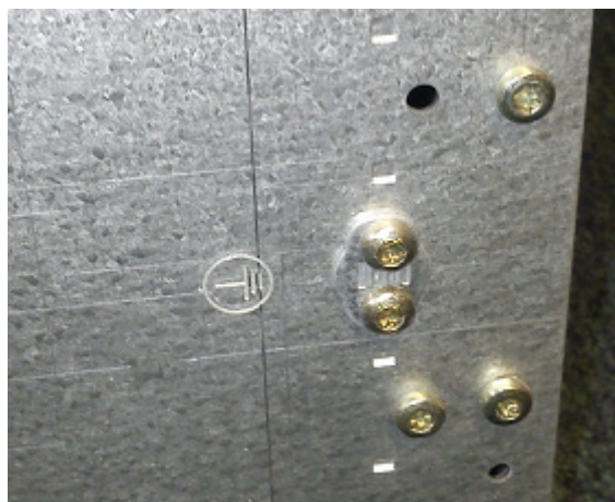
Figure 19: Earthing point 7U-chassis
