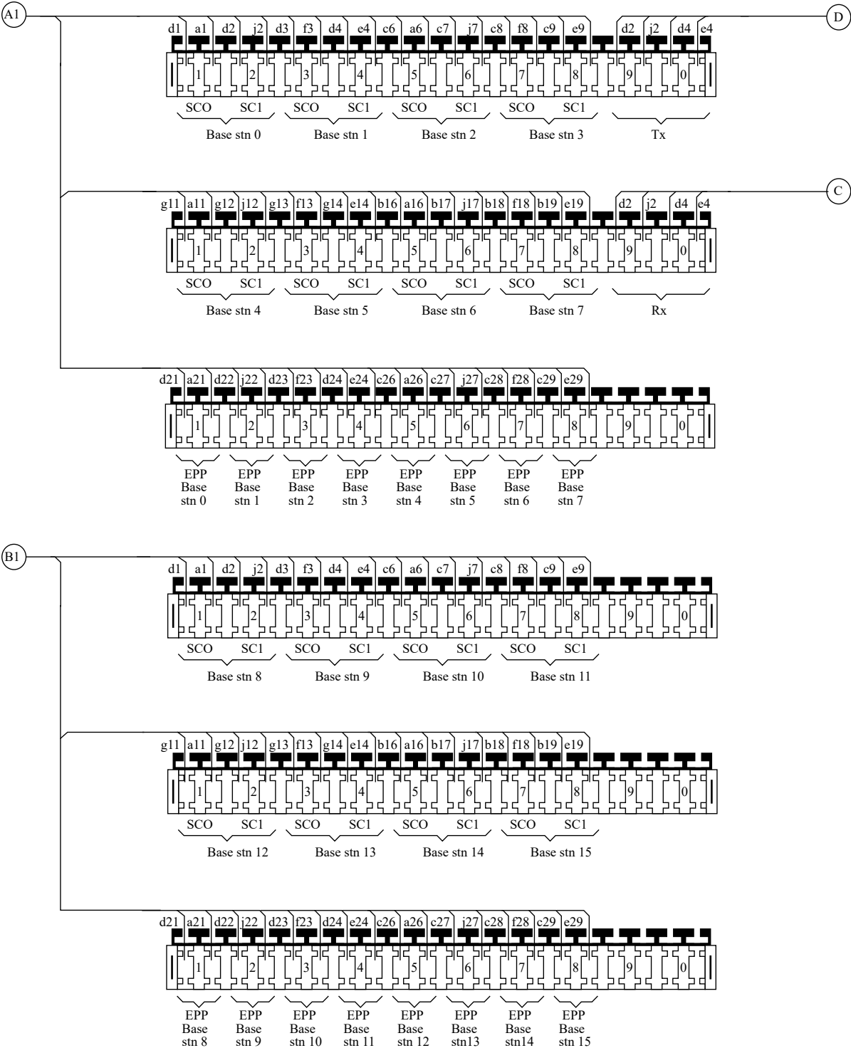
Figure 15: MDF connection of the cables from figure 35 (with EPP)
