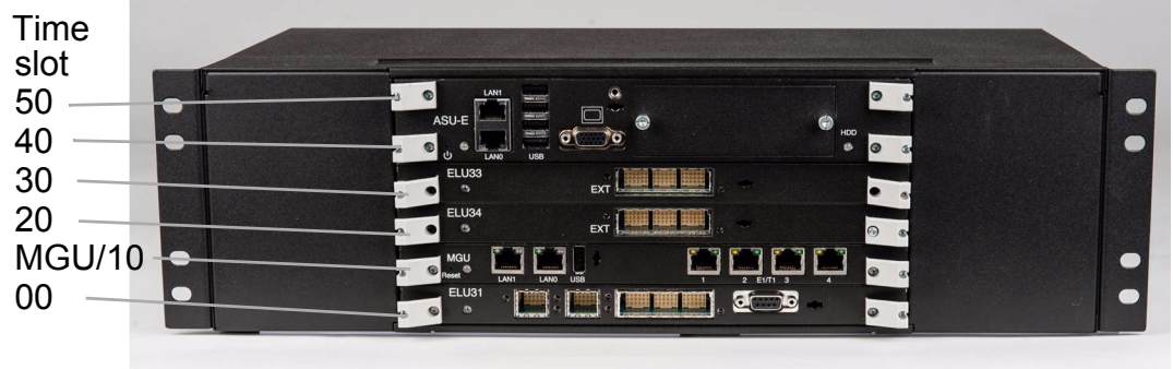
Figure 2: MX-ONE Lite, 87L00039BAA-A, equipped with MGU2, ASU and 3 additional boards
