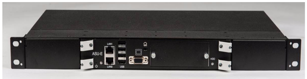
Figure 5: ASU in a MX-ONE 1U chassis
