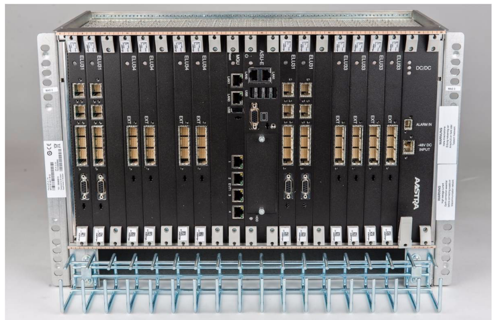
Figure 3: MGU2 and ASU in the 7U high, 19 inch chassis
