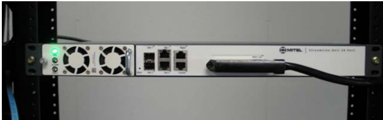
StreamLine 24-Port Model RJ21 Connection
