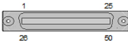
Downlink Port Pinout
