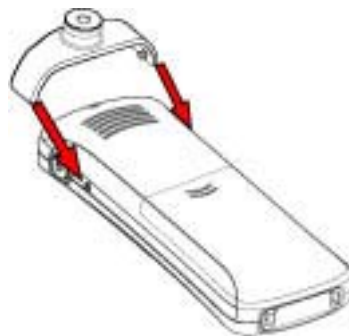
Figure 12: Click the clip into position
