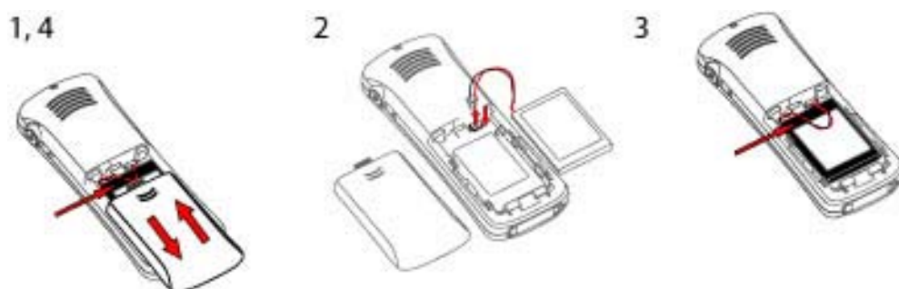
Figure 10: Battery replacement
