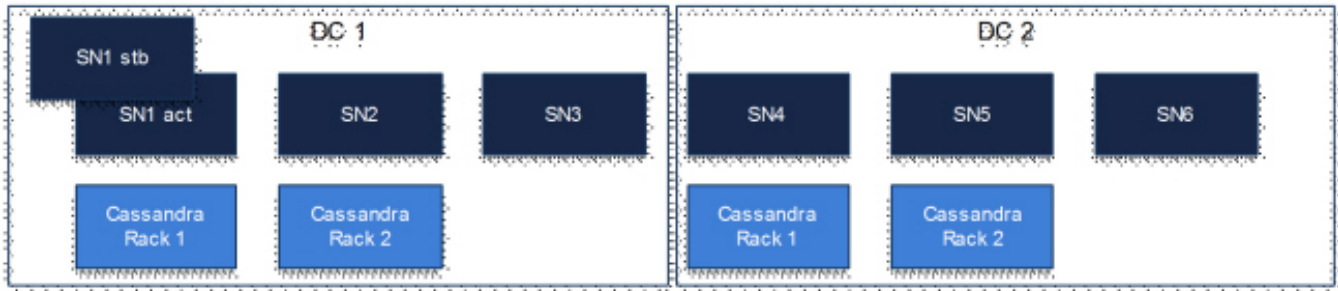
Figure 2.8: Cassandra in multi-site, co-located with the SNs, but only with one Cassandra node per DC. A total of 6 SNs and 6 DCs (geographical locations). No server redundancy.
