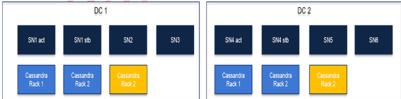
Figure 2.10: Cassandra with 2 DCs (and 2 clusters), where DC2 is remote, and server redundancy is used in both DCs, i.e. SN1 and SN4 have standby servers.
