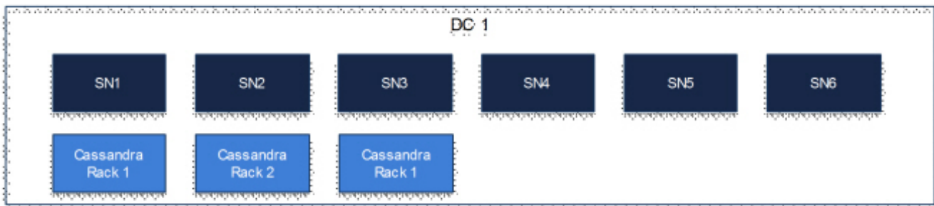
Figure 2.9: Cassandra in single site, the database is standalone (3 nodes). 1 Data Center with 3 racks, and a system with 6 Service Nodes. No server redundancy.
