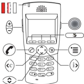
LED Display: On, flashing, off
