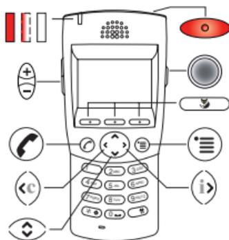
LED display: On, flashing, off
