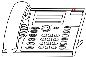
Stand rest; can also be used as a mounting frame for wall mounting
