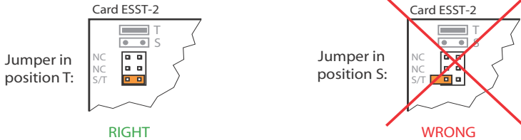
Fig. 24 Jumper position on ESST card
