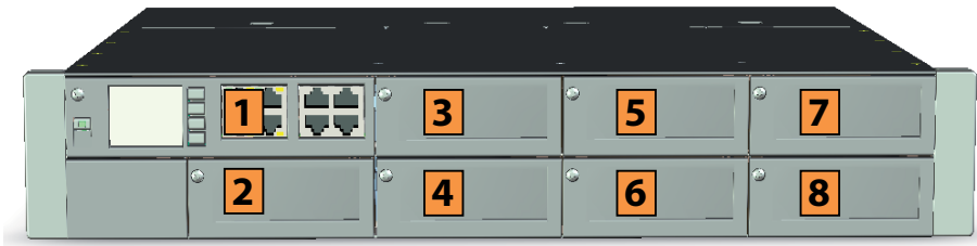
Fig. 26 Number of the Mitel 470 slots
