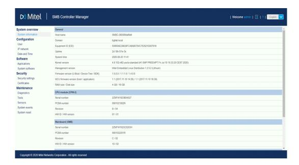
The SMB Controller Manager is included in the file system of each SMB Controller and is part of SMB Controller system software.
