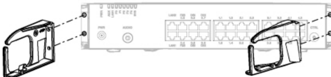
Figure 4.8: Installing the brackets for the cable cover
