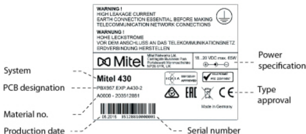
Figure 7.1: Rating plate (example Mitel 430 communication server)
