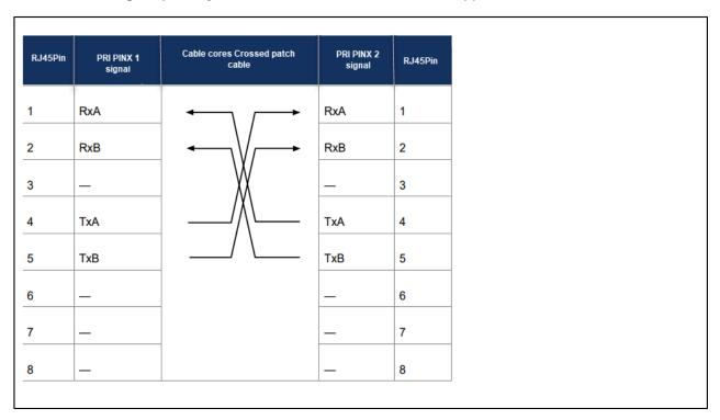
Figure 39: Primary rate interface, networked with transmission equipment
