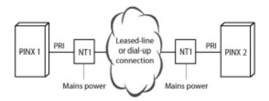
Table 52: Cabling for primary rate interface, PRI, networked with leased-line or dial-up connection
