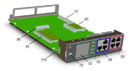
Figure 7: Interfaces, display and control elements of the call manager card CPU1
