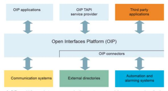
Figure 2: OIP as middleware between communications system, external data sources and applications
