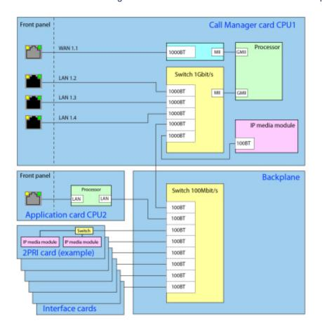
Figure 9: Overview of the Mitel 470 Ethernet concept
