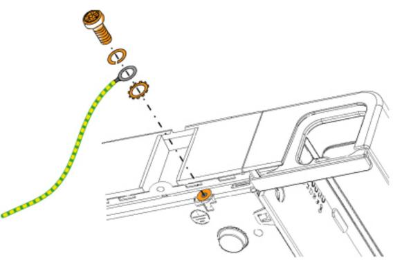
Figure 18: Earthing connection
