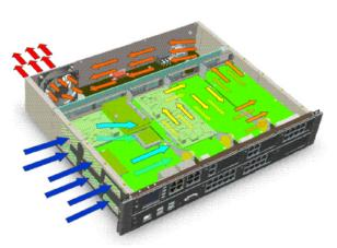
Figure 15: Flow of hot air
