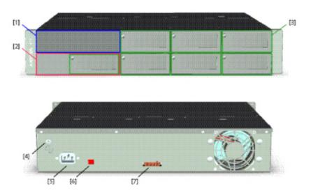
Figure 6: Position of the interfaces on the basic system
