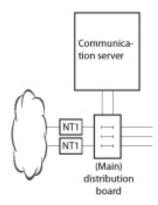
The interface sockets on the front panel and on the fan-out-panel (FOP) where applicable are connected with the (main) distribution frame or the patch panels using either patch cables or prefabricated system cables (see <a href="Equipment Overview"><u>Equipment Overview</u></a>).
