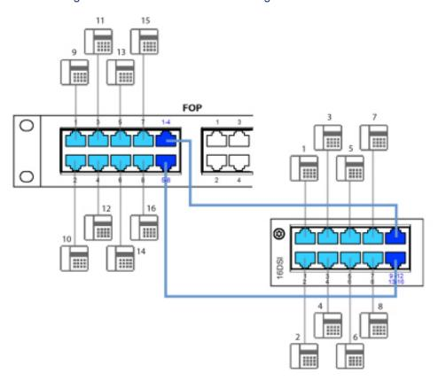
Figure 43: Connection of four-fold assigned sockets via FOP connector strip
