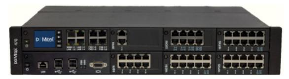
The Mitel 470 communications server ships with a plug-in processor card (call Manager card) with colour display, 4 analogue terminal interfaces and 3 Gbit-LAN connections. A second CPU card (applications card) can be fitted as an option. It contains the pre-installed applications server for unified communications and multimedia services.
