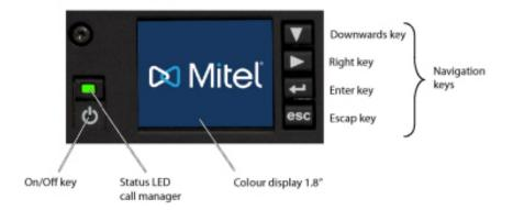
Figure 54: Mitel 470 display and control panel
