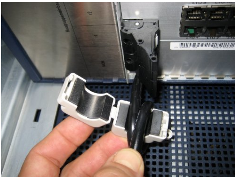
Figure 38: Looping the AC cable through the ferrite core
