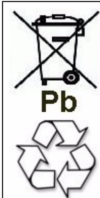
Used accumulators and batteries with this sign are valuable economic goods and must be recycled. Used accumulators and batteries that are not recycled must be disposed of as hazardous waste with full observance of all regulations.
