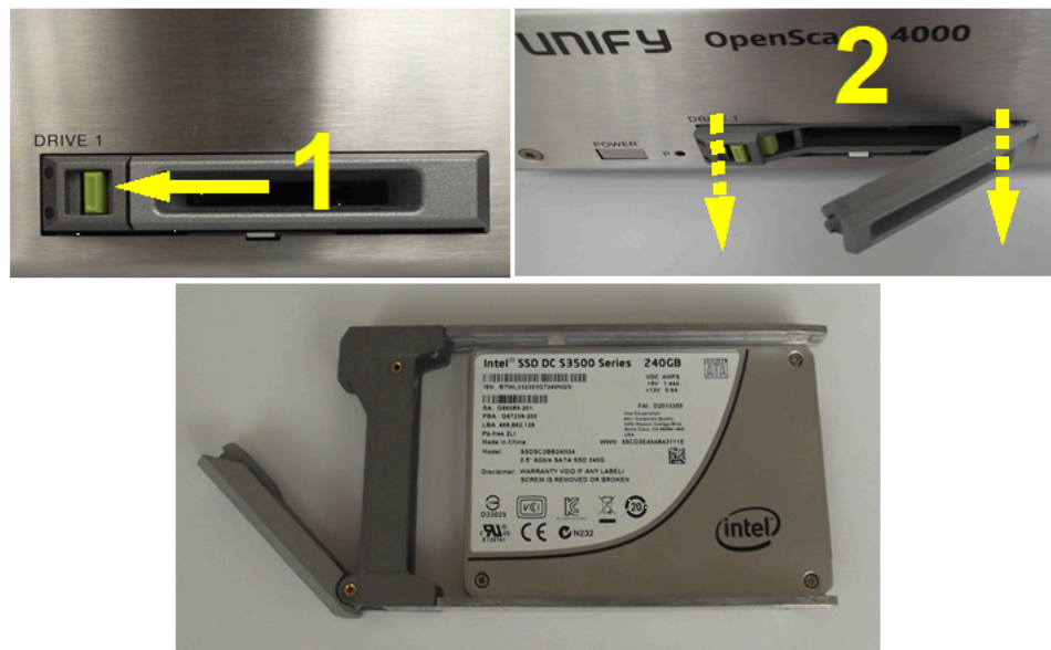
Figure 10: EcoServer: SSD Tray austauschen
