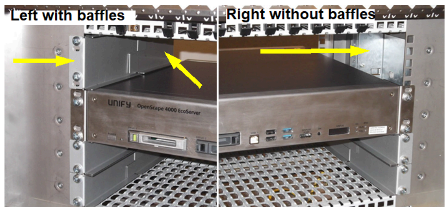
Figure 27: Air baffles above the EcoServer in simplex mode
