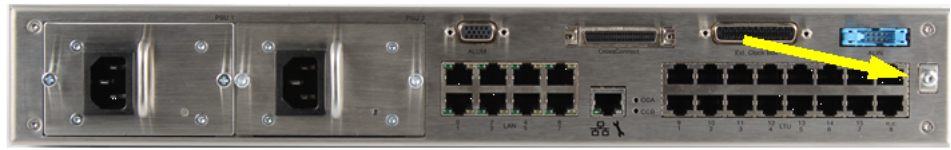
Figure 91: EcoServer - Equipotential bonding conductor
