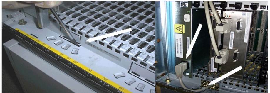
Figure 96: Routing the power cable
