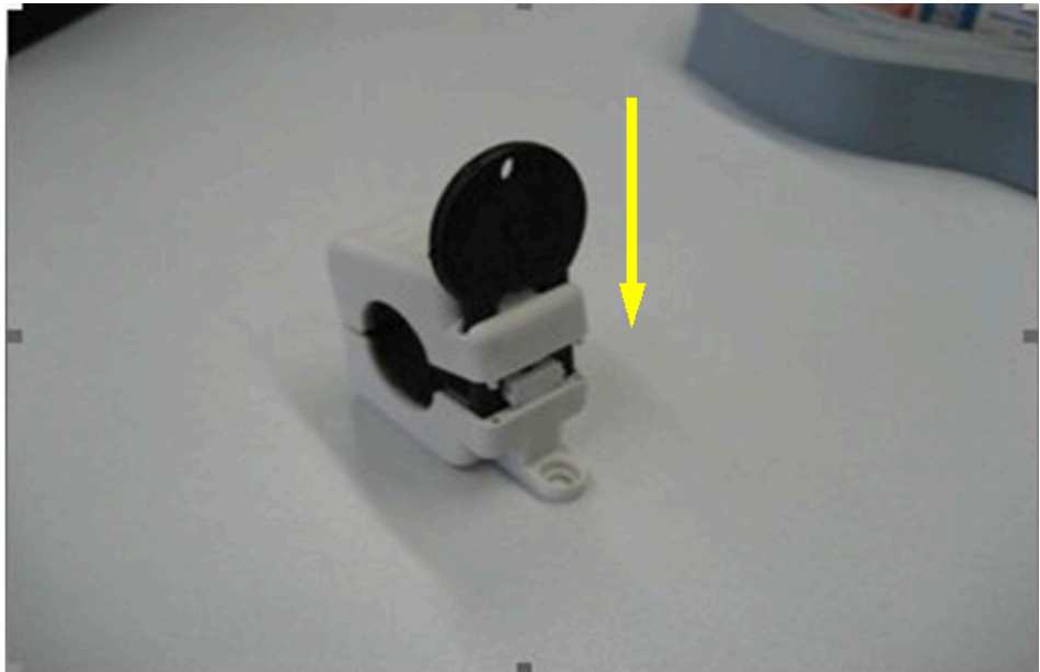
Figure 50: Pressing the key tool into the housing of the ferrite
