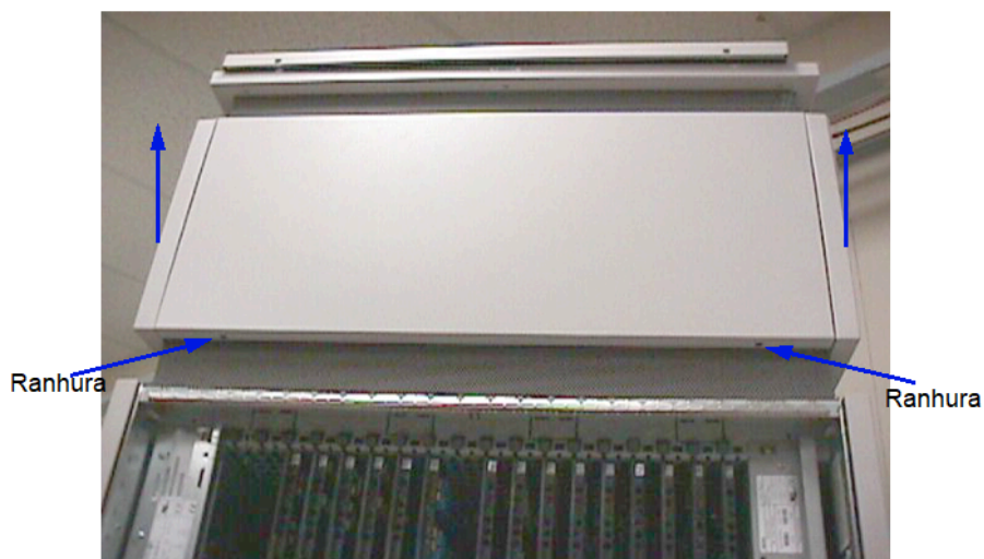
Figura 12: Retirar as tampas frontais 1
