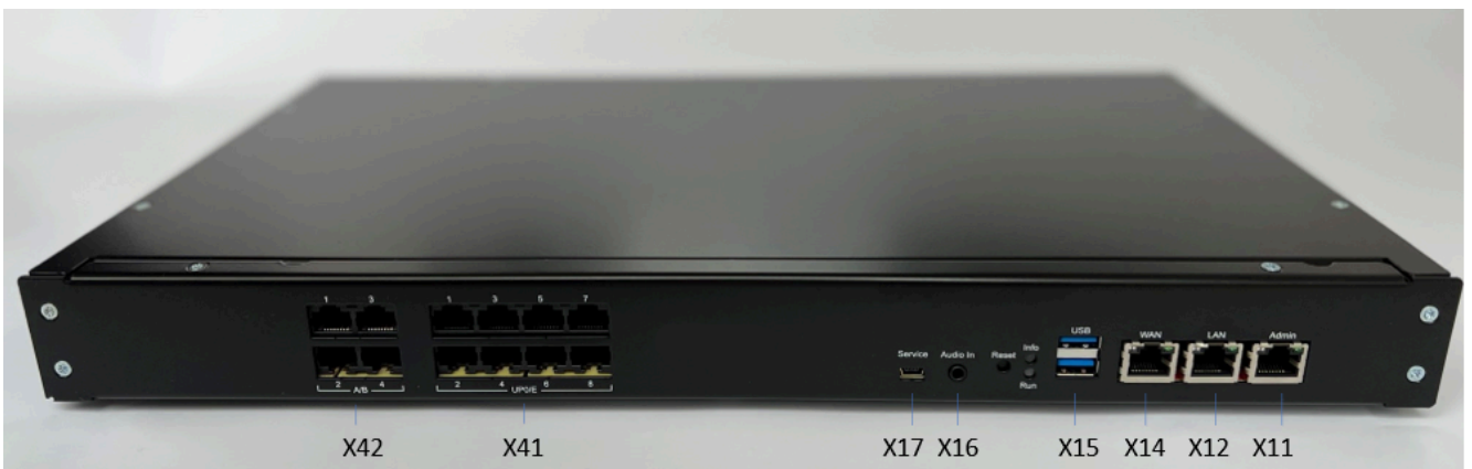
Figure 3: X1R front panel interfaces
