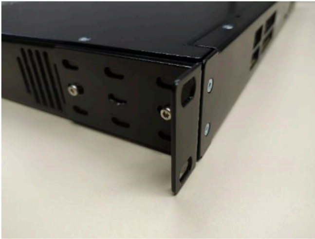
Figure 11: Brackets to fix on vertical rail
