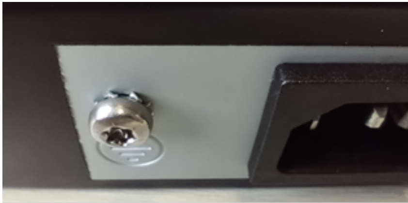
Figure 1: Protective grounding equipment
