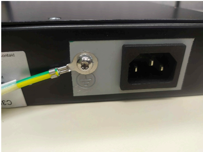
Figure 1: Protective grounding equipment
