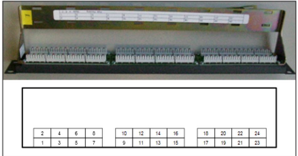
Figure 7: S 0 Patch Panel C39104-Z7001-B3
