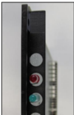
Figure 77: TMEW2 – LEDs on the Front Panel
