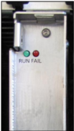
Figure 42: SLCN – LEDs on the Front Panel
