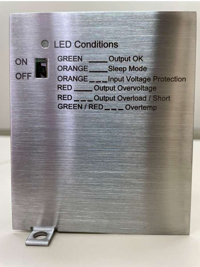
Figure 18: LUNA3 – Front Panel
