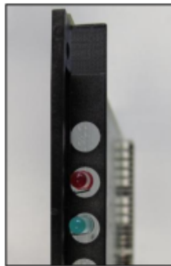
Figure 40: SLMAV8N, SLMAV24N – LEDs on the Front Panel
