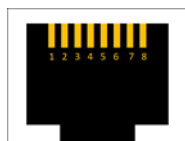
Figure 15: DIUT3 – PIN assignment of RJ45 jack on front panel
