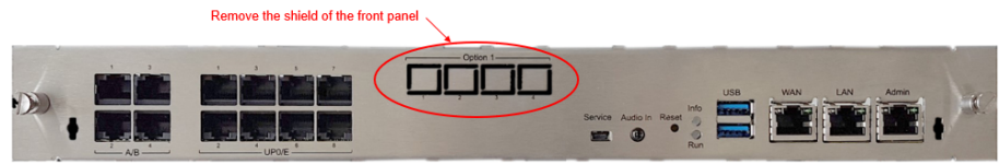
Figure 57: Option 1 position of the OCCMBR or OCCMAR mainboard
