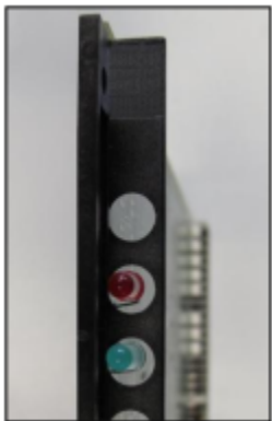
Figura 73: TMDID – LED en la placa frontal
