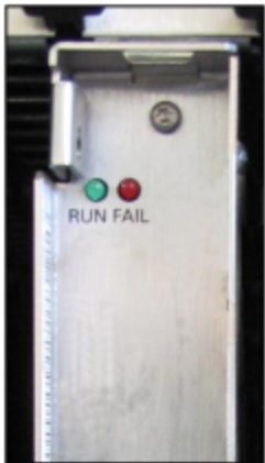
Figura 39: TMEW2 – LED de la placa frontal
