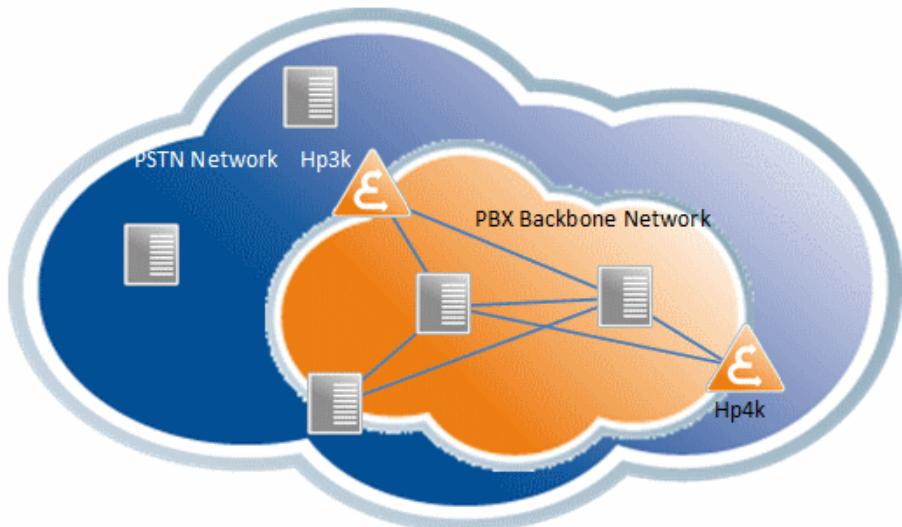
To bring an OSV into an existing TDM PBX network, IP to TDM gateways are added to connect OSV with the TDM PBX. If it needs to integrate with an IP PBX, then an SBC may be needed to connect with the IP PBX. OSV supports connecting directly with the HiPath3000 and HiPath4000 PBX's.
