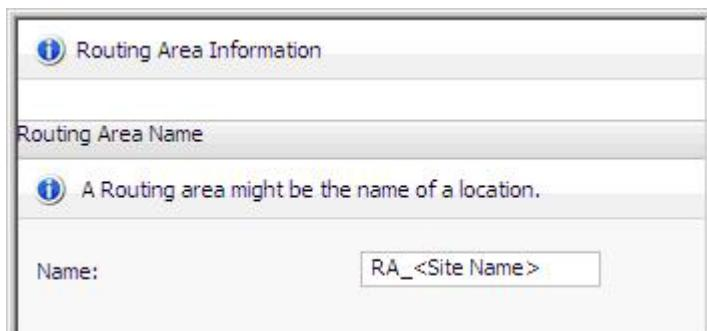
The routing area will be used as location identifier for a site. Every subscriber and endpoint of the site will receive the site's routing area.
