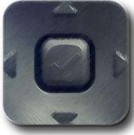
UI navigation is easily performed using the navigation keys located to the right of the LCD screen. The Left and Right navigation keys are used to switch to the different screens and the Up and Down keys are used to highlight and scroll through the different lines/calls on the respective screen. The figure below provides a visual representation of the different screens and the UI behavior when a navigation key is pressed.
