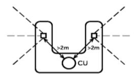
The length of the extension microphone cable is up to 8 ft (2.5 m).
