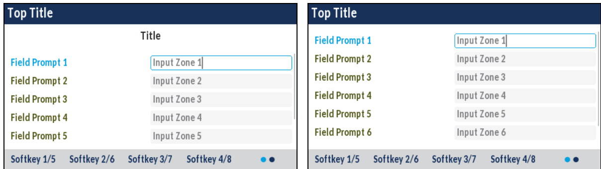
Figure 59: InputScreen implementation on 6930 “condensed” mode
