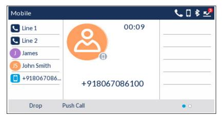
Lift the handset or press the key, blinking Bluetooth Line key, or Answer softkey for handsfree operation.
