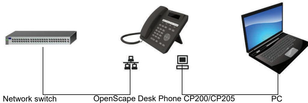
Using this connection option saves one network port for each switch used and allows shorter network cables to be used when arranged correctly.
