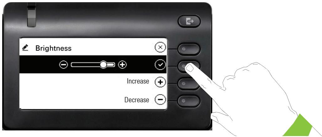
Complete the setting by pressing the Softkey for **✓**.
