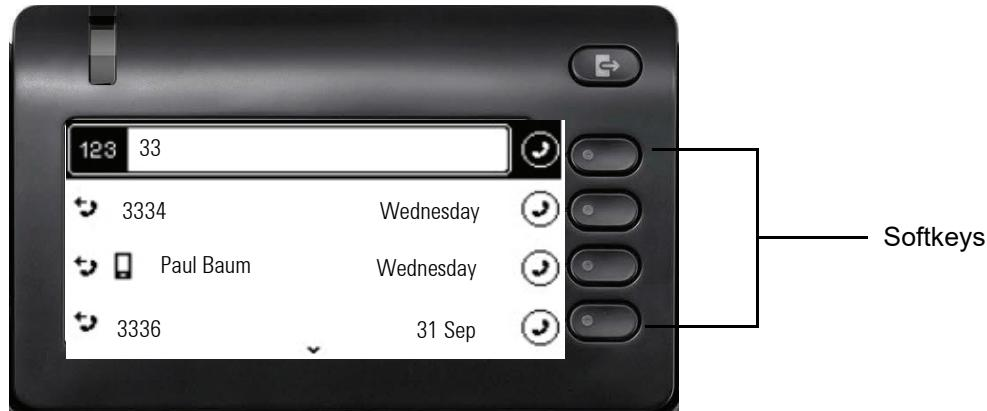
As soon as you enter the first digits, an input field opens for selecting the phone number and you will be shown conversations that match the input to date in the corresponding positions.
