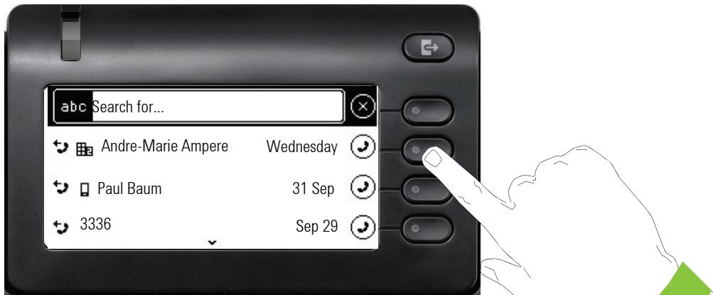
Use the Softkey to dial the respective subscriber. You can choose a conversation beforehand using the Navigator keys  $\blacktriangleleft$  and  $\triangleright$  and open the details of the conversation with the  $\blacktriangleright$  key → page 34.
