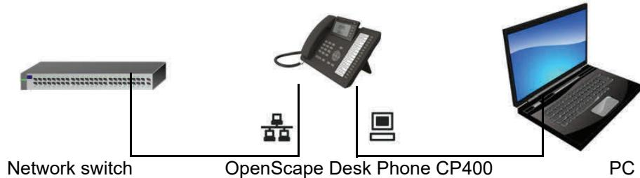
Using this connection option saves a network port for the switch used and allows shorter network cables to be used.
