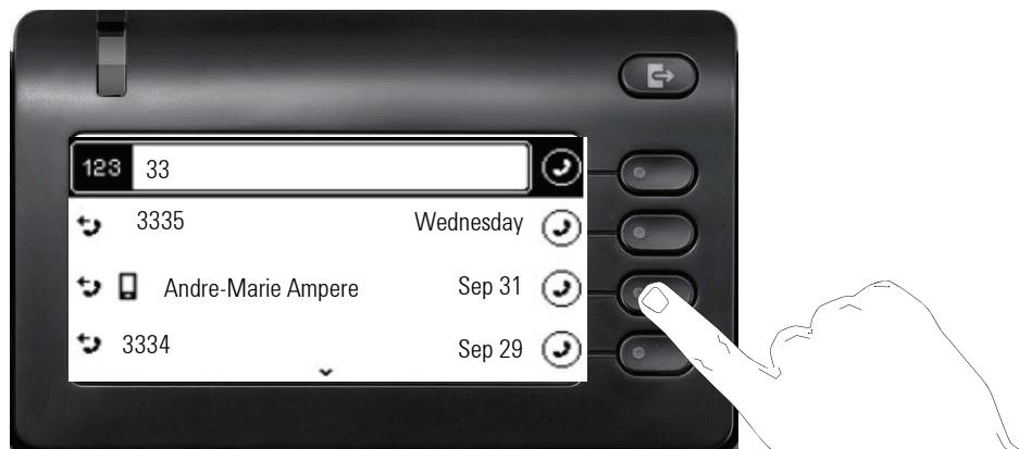
Use the **#** key to switch from numeric to alphanumeric input when you have opened the search field with the Softkey
