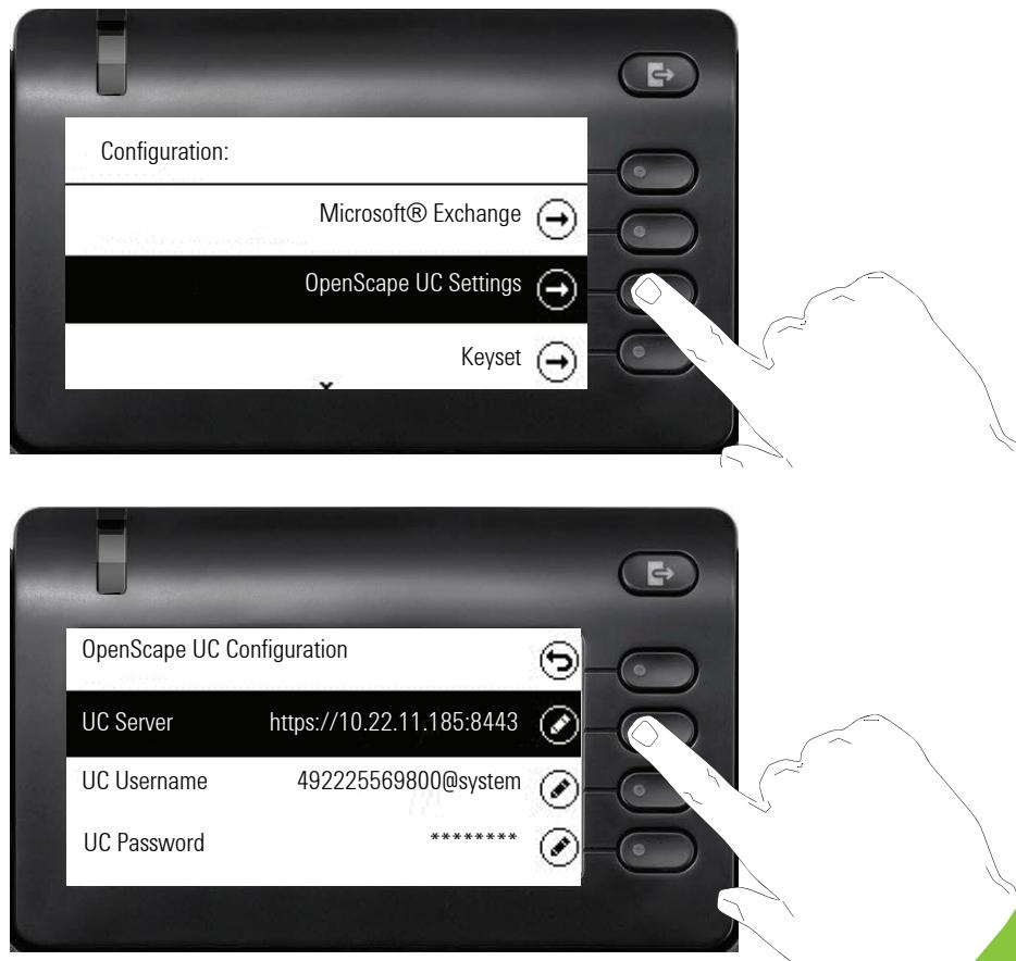
The OpenScape CP400 will login using the given user credentials. If the data is incomplete (missing server address, username or password) the phone will not try to login at all.
