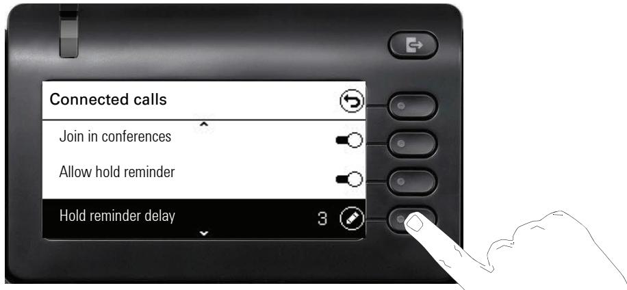
Press the Softkey for to open the setting.
