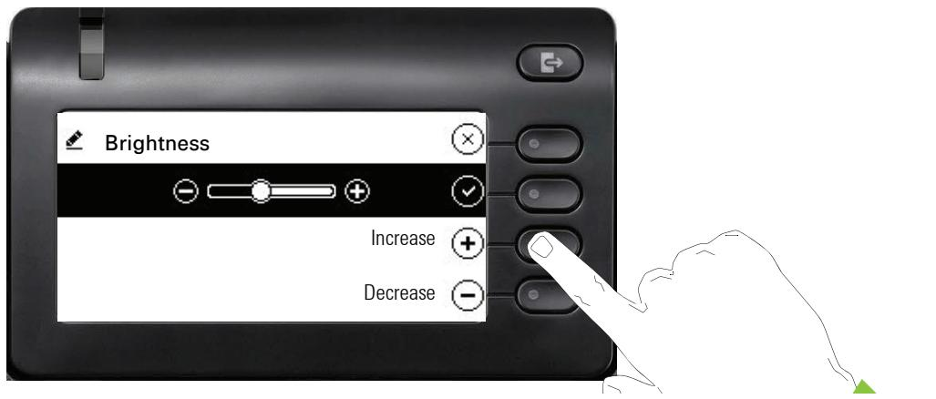
Adjust the brightness to the desired level. Use the **- +** key to do this. The display is adjusted immediately.
